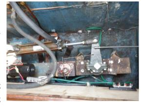
is controlled through wheels at both helms, through approved copper lines and flexible hose, bronze rudder with stainless steel rudder post and bronze tiller arm. Post is supported on hull bearings that incorporated standard bronze packing gland and top collar bearing supported in an alloy shelf. As much as possible all components were inspected and found to be in good order. System fitted with a VDO rudder position indicator.
