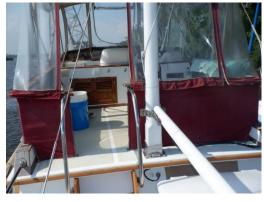
center. Pedestal helm seat, companion seating over storage pods, cushions with cracking vinyl from sun exposure. Stainless steel aft rail is well secured with teak stairs provided aft.
