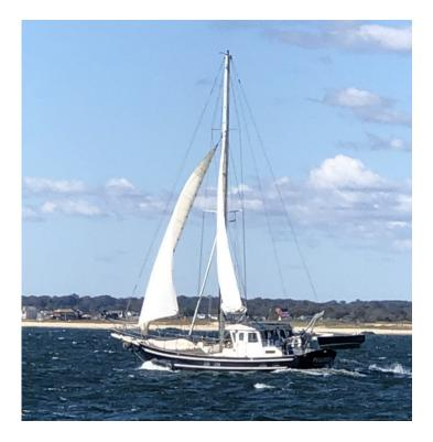
Pegasus has Agantyr's single-stick "schooner" rig, scaled to her smaller dimensions. Her LWL is 36 ft, LOD 45 ft, Beam at sheer 13 ft, draft 4' 6", tandem centerboards, 25 tons displacement, 1200 sqft working rig consisting of 450 sq ft #1 Yankee, 350 sqft #1 staysail, 400 sq ft Main. 1200 sq ft cruising chute, 700 sq ft tri-radial drifter, She comes with a cruising chute with sock, tri-radial drifter, nos 1, 2,
